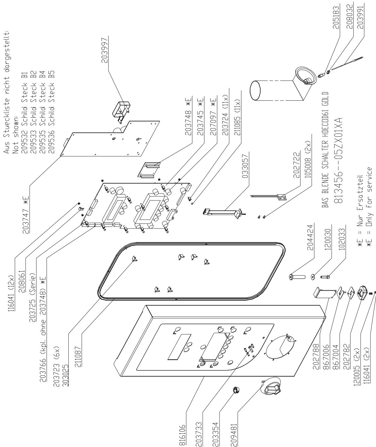
Until S/N 09021471 with serial port #033023 instead of USB port
