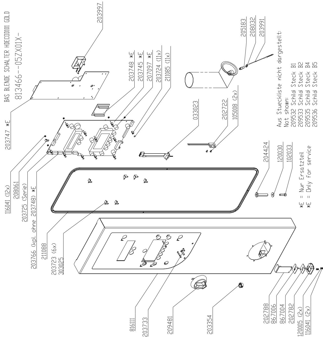
Until S/N 09021471 with serial port #033023 instead of USB port
